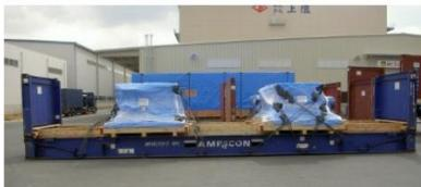
Solid chocking composed by lumber as sufficient bracing should be installed in order to prevent sliding shipments during sea going. The chocking should be reached from end panels to shipments tightly.
