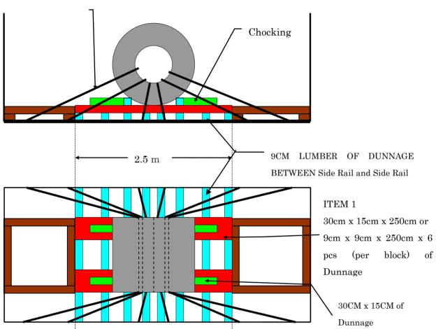
THIS IS THE VANNING PLAN, WHICH IS CONSIDERED SAFE NAVIGATION FOR STEEL COIL SHIPMENT.
